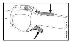
Press down the throttle trigger lockout and open the throttle – the choke knob moves to the run position I. After a cold start, warm up the engine by opening the throttle several times.
