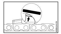
File the top of the depth gauge parallel to the stamped service marking (see arrow) – but do not lower the highest point of the depth gauge in this process.
