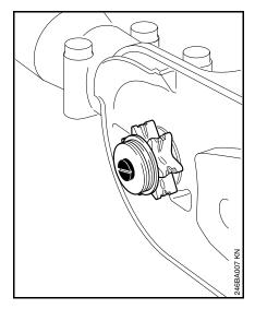
The chain sprocket is driven via a friction clutch. Have the chain sprocket replaced by a servicing dealer.
