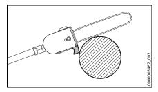
To avoid pinching the bar in the cut, position the cutting attachment with the hook against the branch and then perform the cross-cut from the top downwards.
