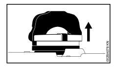
Remove the tank cap.
