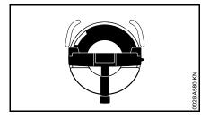
The marks on the cap and oil tank are then in alignment.
