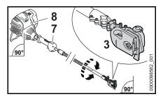
Align the housing (8) (with the manual fuel pump facing up), the control handle (7) (with the stop switch facing up) and the transmission (3) (with the oil tank cap facing up) as shown
