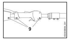
Tighten down the screws (9) firmly
