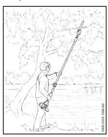
The machine's long reach makes it possible to prune branches that are overhanging obstacles, such as rivers or lakes. The tool angle in this case depends on the position of the branch.
