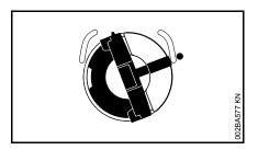
Marks on tank cap and oil tank must line up.
