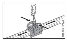
Squeeze the clip (carrying ring) together to move it up or down the shaft.
