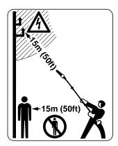
Do not allow other persons within a radius of 15 m of your own position due to falling branches and ejected wood particles – **Risk of injury!**
