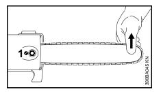
Re-tensioning during cutting work:
