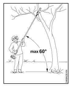
Hold the power tool at an angle. Do not stand directly underneath the limb being cut. Do not exceed an angle of 60° from the horizontal. Watch for falling wood.
