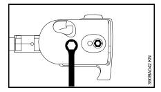
Unscrew the nut and remove the cover.
