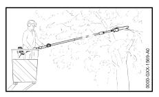
The machine's long reach enables cutting to be performed next to the trunk without the risk of the lift bucket damaging other branches. The tool angle in this case depends on the position of the branch.
