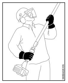
Always hold the power tool **firmly with both hands** – right hand on the control handle, left hand on the drive tube – even if you are left-handed. Wrap your thumbs firmly around the control handle and shaft.
