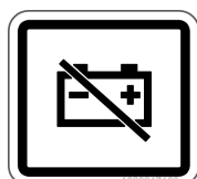
Fig. 21: Battery master switch
