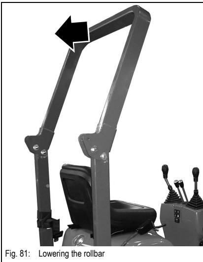
Fig. 80: Lowering the rollbar
