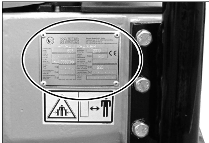
Fig. 1: Type label: location (symbolic representation)
