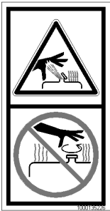
Fig. 26: Reservoir under pressure
